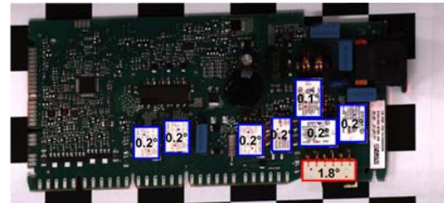
(b) Inspection results for a defected board
