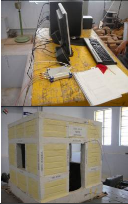
Fig. 9 Instrumentation and location of Accelerometers
