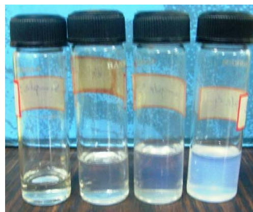
Fig. 4 Photographs of prepared nanoemulsions with Tergitol 15-S-5, Tergitol 15-S-7, Tergitol 15-S-9 and Tergitol 15-S-12 (From left to right)
