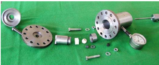
Fig. 2 Dismounted jig for the head destructions
