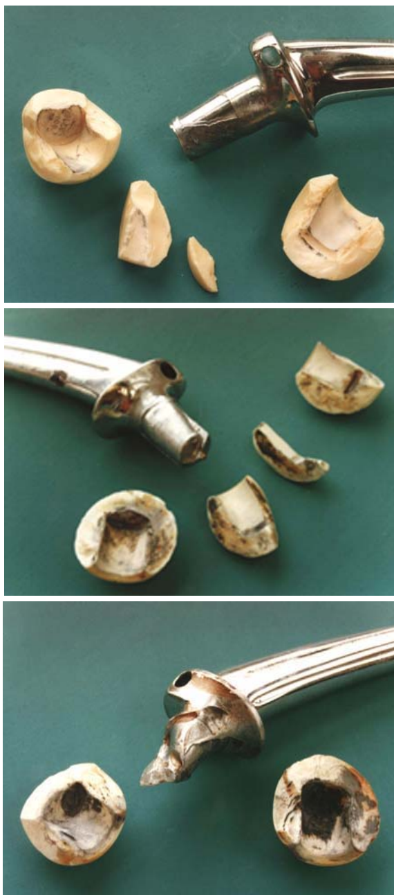
Fig. 1 In vivo destructed ceramic heads
