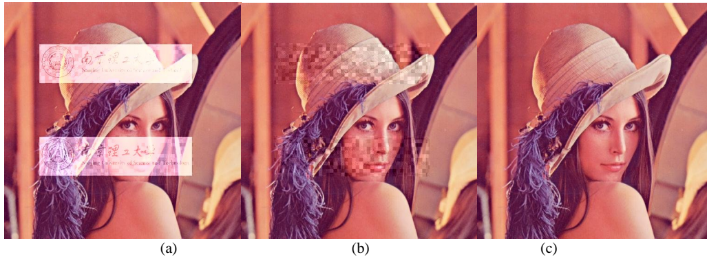
Fig. 5 Results for a = 0.5 , c = 0.6 and d = 0.8 : (a) Watermarked Image (Psnr: 15.2), (b) Remove without Right Key (Psnr: 22.4), (c) Remove with Right Key (Psnr:56.8)
