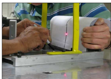
Fig. 1 Laser beam adjustment with collimator device
