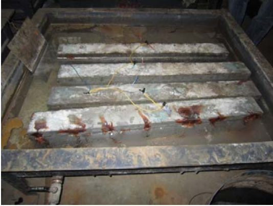
Fig. 3 Accelerated Corrosion Process for Unstressed Condition
