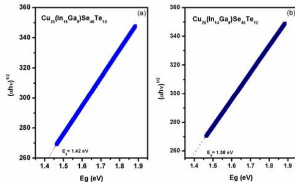
Fig. 5 (a, b). Optical energy band gap ( $E_g$ ) for the CIGST-1 and CIGST-2 alloys
