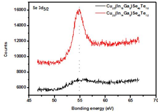
Fig. 2 (b). Se 3d<sub>5/2</sub> XPS core levels spectra for the CIGST-1 and CIGST-2 compositions
