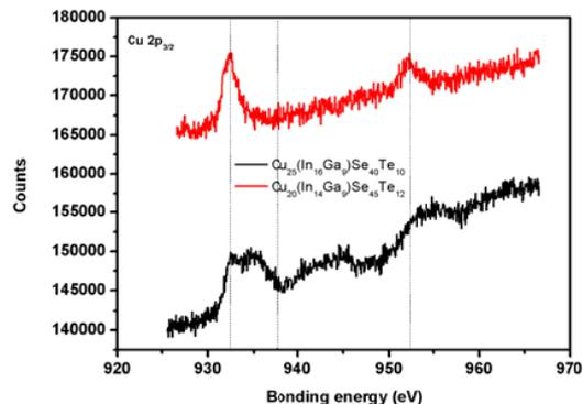
Fig.2 (c). Cu 2p<sub>3/2</sub> XPS core levels spectra for the CIGST-1 and CIGST-2 compositions
