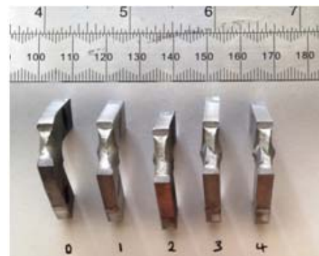
Fig. 11 Fracture surfaces of commercial pure Al before and after ECAP process as a function of pass numbers
