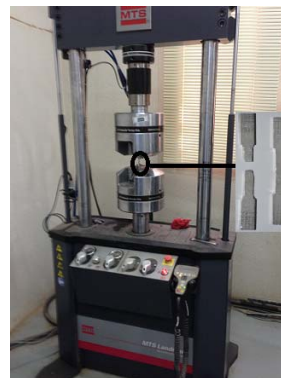
Fig. 2 Commercial pure aluminum sample during tensile test
