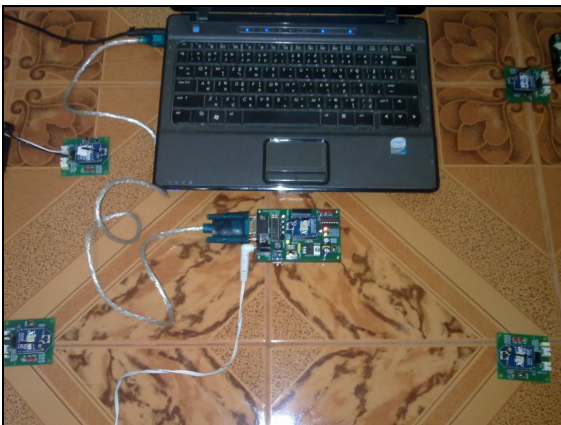
Fig. 4 Equipment used in the experiment: the referencing nodes and the object node
