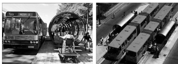
Fig. 4 Tube elevator for special needs users in Curitiba
