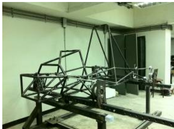
Fig. 20 Rapidamente's torsional stiffness test rig
