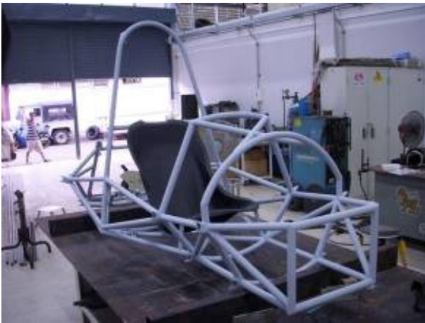
Fig. 14 Rapidamente92 student formula frame
