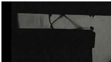
Fig. 6 Schlieren flow visualisation for PR=0.57 and flat tip model
