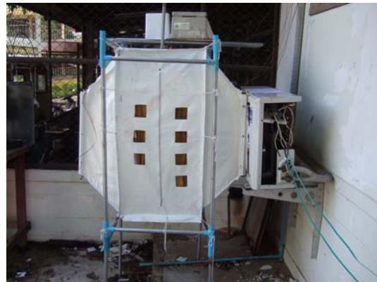
Fig. 9 The drying chamber without auxiliary fan unit
