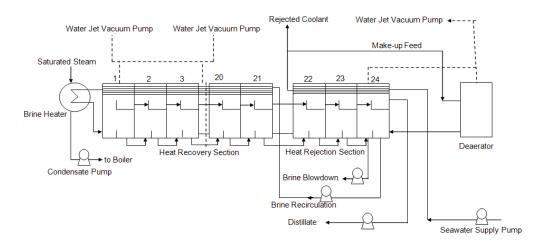
Fig. 2 Schematic diagram of the MSF desalination plant with 24 flashing stages
