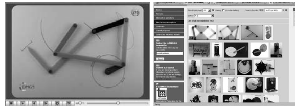
Fig. 6 Physical model digitized and available as video and animation in the DMG-Lib internet portal www.dmg-lib.org (left), picture gallery to support visual image retrieval (right)
