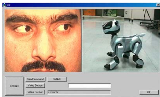
Fig. 9 Eye tracking command to motivate Aibo to start walk
