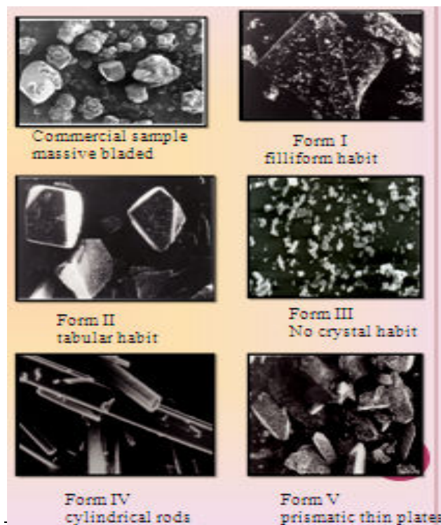
Fig. 1 Scanning electron micrographs of artesunate and its crystal modifications
