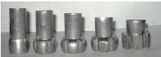
Fig. 14. Teeth formation stages for 3 and 6 teeth parts
