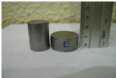
Fig. 2. Initial and final compressed lead specimen
