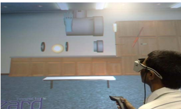
Fig. 8 In a semi-immersive virtual environment, assembling the valve using head, wand and ultra sonic trackers
