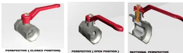
Fig. 3 Different Views of a Ball Valve modeled in AutoCAD
