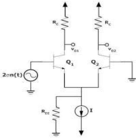
Fig. 1. Differential amplifier with one end grounded
