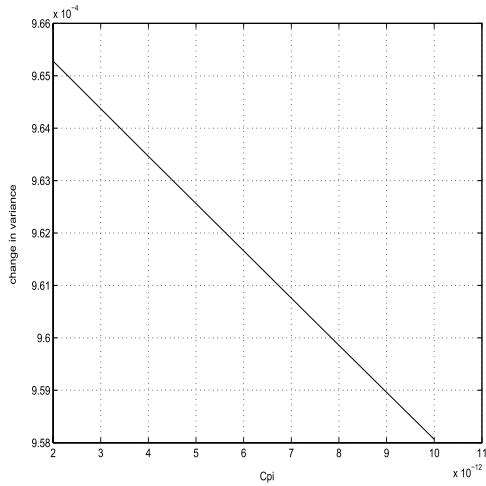
Fig. 6. Effect of device parameter  $C_{\pi}$
