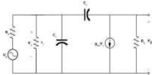
Fig. 2. High-frequency equivalent half-circuit
