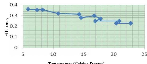
Fig. 6 Systemic Power Efficiency of the Microwave heating system as function of the rising temperature measured as 5 liter of the water was heated in lab-made system
