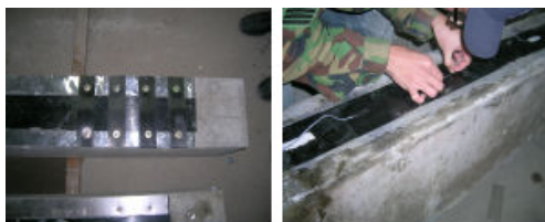
Fig. 6 Intermediate laminates and LVDT setup
