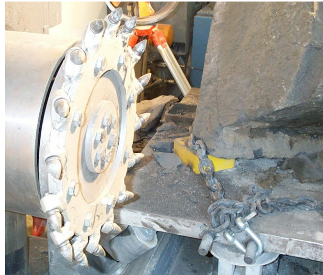
Fig. 8 Typical example of mechanical interaction between bits and hard rock (ore disintegration process)
