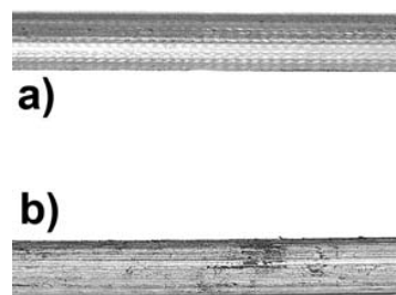
Fig. 2 Surface of 6061+10% vol. SiC composites rods, a) after 3 h preheating; b) after 0.5 h preheating
