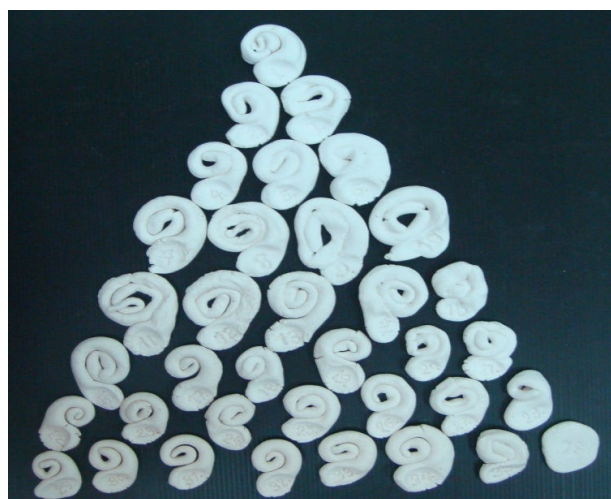
Fig. 6 Color of ceramic body after being fired at 1,230 degrees Celsius
