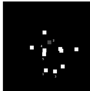
Fig. 5 Test data cube. Objects 1 and 2 have parallel trajectories ( 240^\circ ) and the same velocity amplitude ( 1/3 ). Object 3 has velocity 255^\circ , 1/4 . Object 4 is accelerating with direction 240^\circ . Object 5 is moving on a circle
