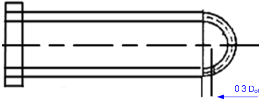
Fig. 6 Tube Length Definition for U-Tube [8]
