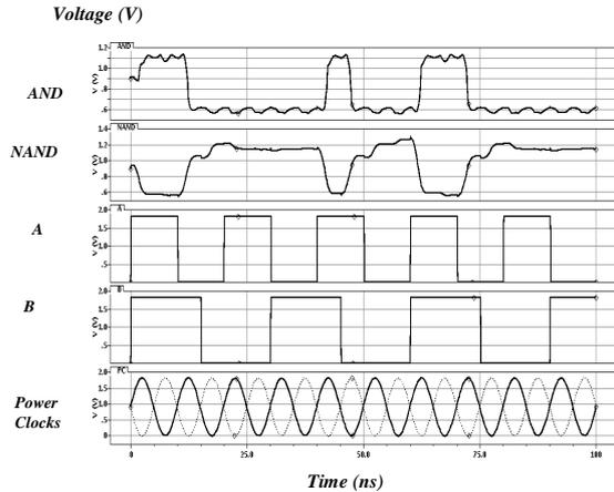
Fig. 2(b) Simulated CEPAL NAND gate timing waveforms
