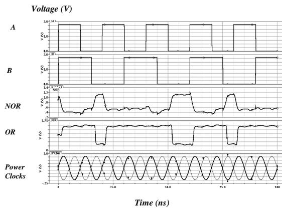
Fig. 3(b) Simulated CEPAL NOR gate timing waveform
