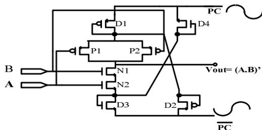
Fig. 2(a) CEPAL NAND gate schematic diagram
