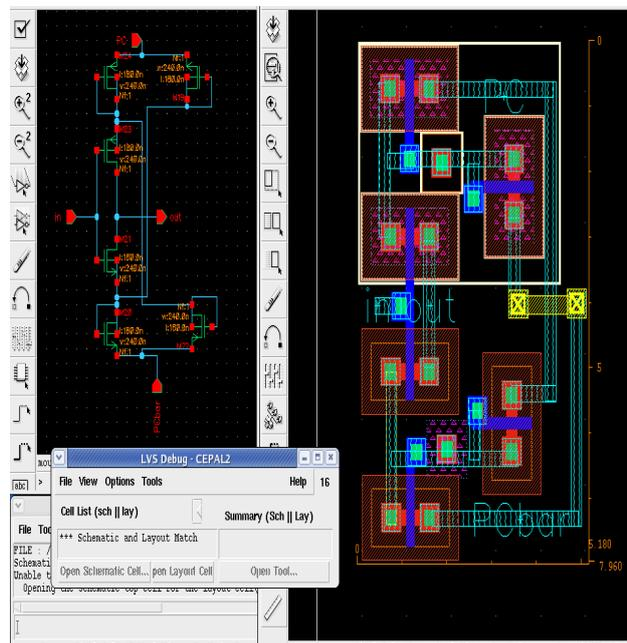
Fig. 11 Layout of a CEPAL inverter circuit
