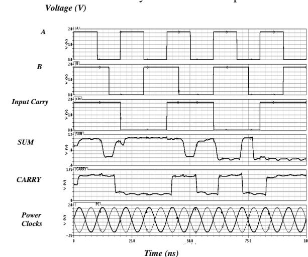
Fig. 7(b) Simulation waveforms of CEPAL full adder
