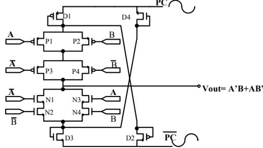
Fig. 4(a) CEPAL XOR gate schematic diagram
