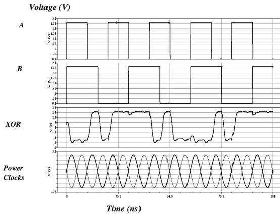
Fig. 4(b) CEPAL XOR gate simulated timing waveforms
