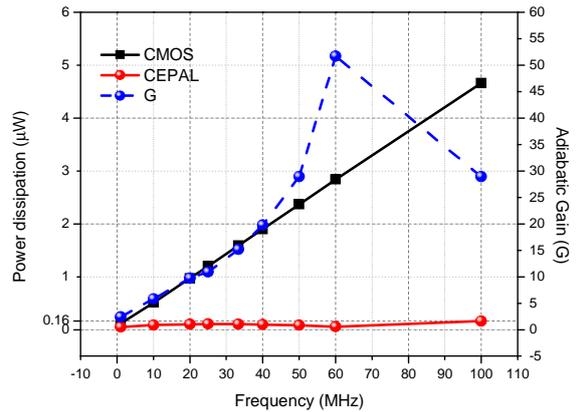
Fig. 8 Power dissipation per cycle and adiabatic gain versus operating frequency (at  $f_{PC}/f_{in}=2$ ,  $V_{DD}=1.8V$  and  $C_L=10fF$ )
