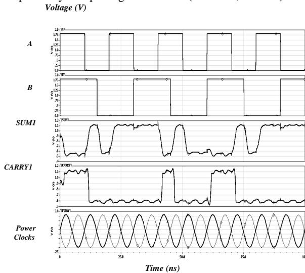
Fig. 7(a) Simulation waveforms of CEPAL half adder
