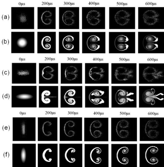
Fig. 1 Multiple dynamics images and numerical simulation results by MVFT at  $t=200, 300, 400, 500, \text{ and } 600 \mu\text{s}$  after shock passage. [The experiments corresponding (a), (c), and (e), and the simulations corresponding (b), (d), and (f)]
