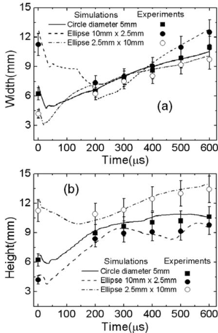
Fig. 3 Comparison of the width and height between the experiments and simulations. (The error bars of this visual measurement are equal to  $\pm 10\%$ )
