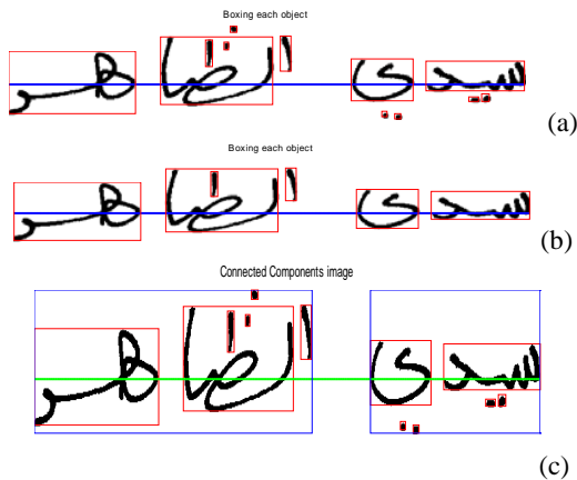
Fig. 2 Examples of extracted connected components (a), sub-words of combined components (b), and detected words (c)
