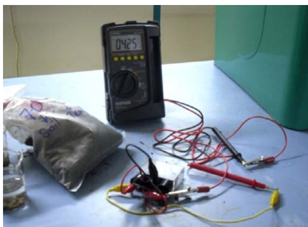
Fig. 3 Three series of compacted vermicompost produce 4.25V
