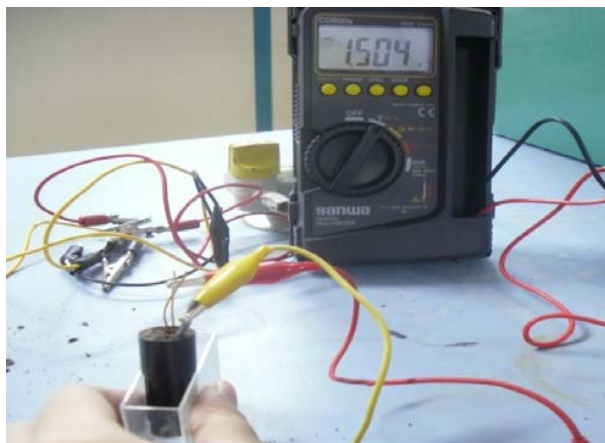
Fig. 2 One series of compacted vermicompost produces 1.504V
