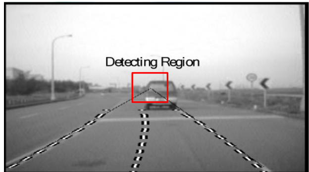
Fig. 2 Software result of lane detection
