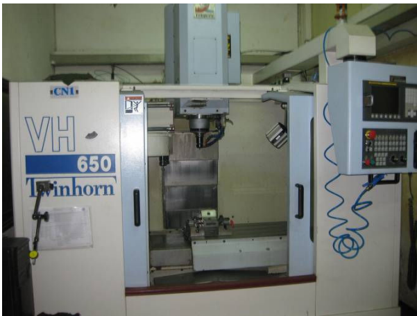
Fig. 3 CNC high-speed milling machine 'Twinhorn VH650'
