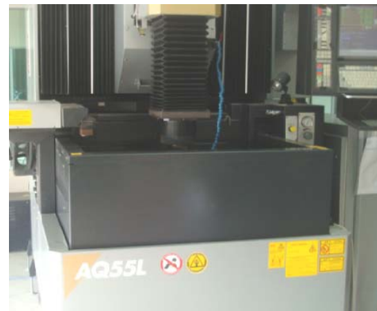
(b) EDM tank with electrode and workpiece.
