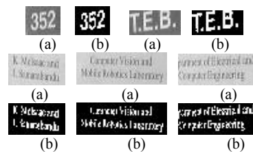
Fig. 11 Test image showing both dark and light text (a) Sub-Images (b) Extracted text Strings
