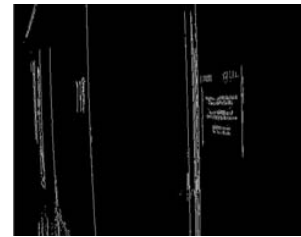
Fig. 5 Resultant vertical edges by combining strong and weak edges
