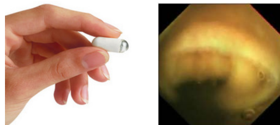
Figure 1 Wireless Capsule Endoscope (WCE) and an example image taken
