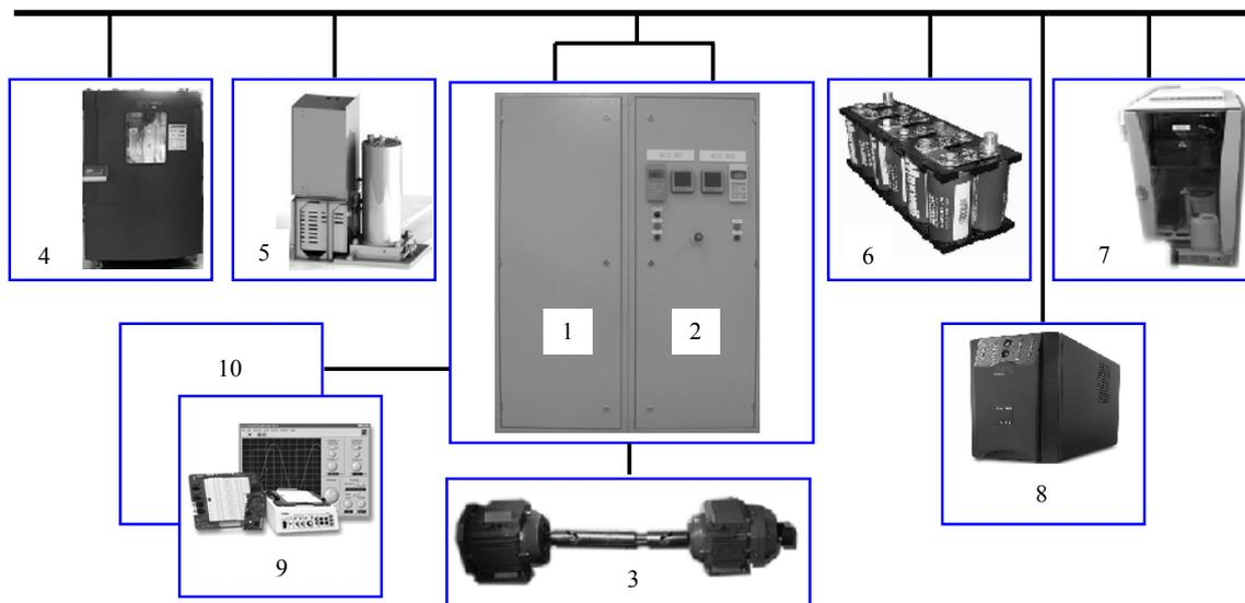
Fig. 1 Setup composition: 1 – Prototype of the propulsion electric drive; 2 – Loading electric drive; 3 – Prototype of the mechanical transmission; 4 – Traction battery; 5 – Flywheel energy storage; 6 – Supercapacitor storage; 7 – Fuel cell; 8 – UPS; 9 – LabView software and corresponding hardware; 10 – Measuring devices and instruments
