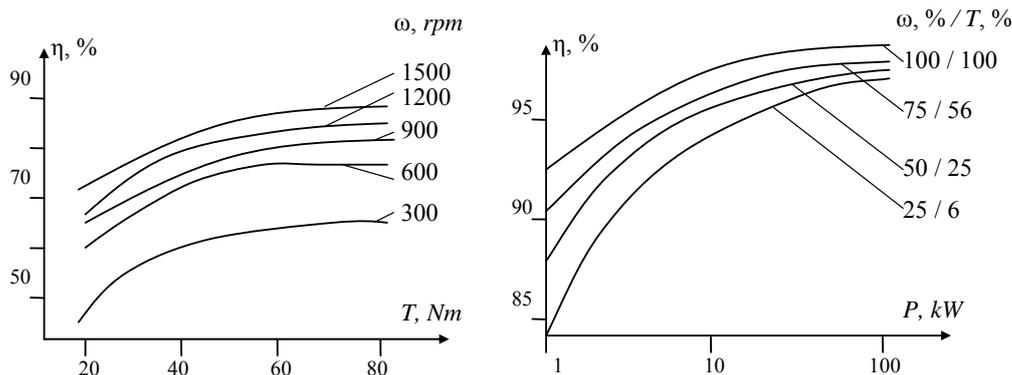
(a) Impact of rotational speed ( $\omega$ ) and load torque ( $T$ ) on efficiency ( $\eta$ ) of a 2.2 kW induction motor driven with a frequency converter
