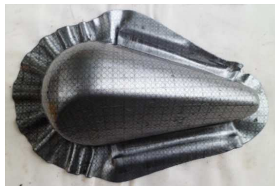
Fig. 12 Workpiece with grid to measure the strain
