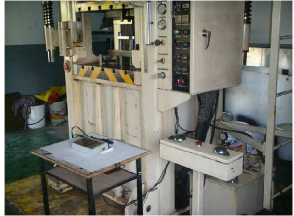
Fig. 7 Installation of the device for oil pressure measurement to the hydraulic press
