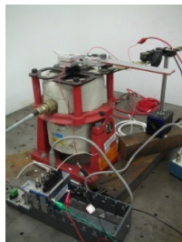
Fig. 14 The experimental photograph for the ERF TVA testing setup
