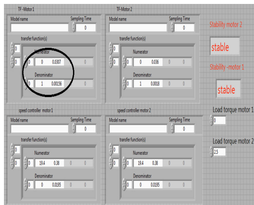
Fig. 8 Front panel representation for stability analysis of parallel connected induction motor drive for 25% increase in stator resistance of motor 1
