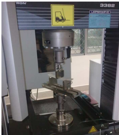
Fig. 5 Experimental setup for ENF Test
