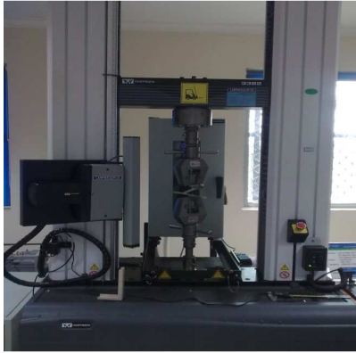
Fig. 4 Experimental set up for DCB Test
