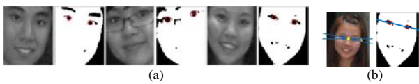
Fig. 13 (a) eyes location using Hough circle detection; (b): illustration of face angle measurement
