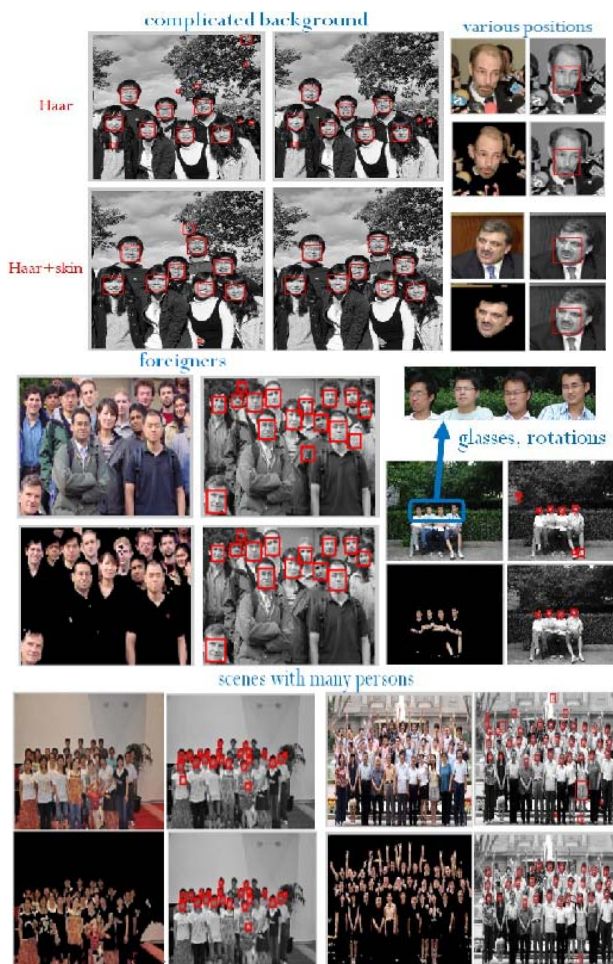
Fig. 25 Some results showing the performance of Haar-like face detection versus Haar with skin color segmentation based on photographs with variously situated faces
