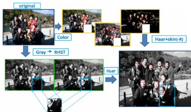
Fig. 12 Scheme of our proposed method—RHST+Skin(-R) (combination of Haar-like face detection, skin segmentation and RHST)
