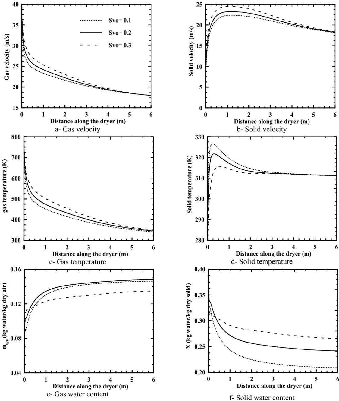
Fig. 10 Effect of inlet velocity slip coefficient,  $S_{vo}$ , on the axial distribution of velocities, temperatures and water content along the dryer for both phases.
