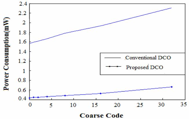
Fig. 5 Power consumption of the two DCO structures
