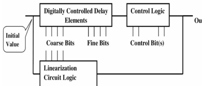
Fig. 1 Block diagram of the ring oscillator DCO
