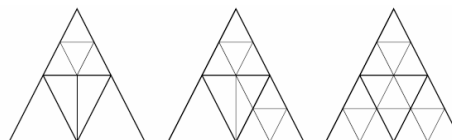
Fig. 3: (a) one subdivided neighbor triangle (b) two subdivided neighbor triangles (c) regular subdivision [14]
