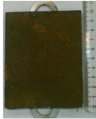
Fig. 3 Grade of Rust of specimen surface "C" according to ISO 8501
