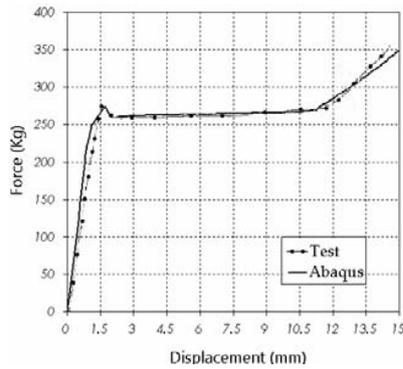
Fig. 2 PVC loading in uniaxial with velocity 2mm/min
