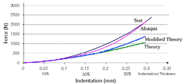
Fig. 9 Indentation in 2layer laminate with 10mm indentor
