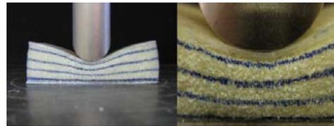
Fig 12 Indentation in sandwich beam with PU core
