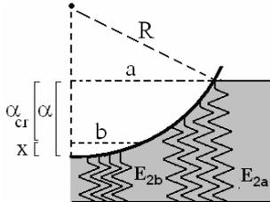
Fig. 5 Two modulus consideration for laminates indentation
