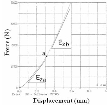
Fig. 3 Lateral compression in 4layer composite laminate
