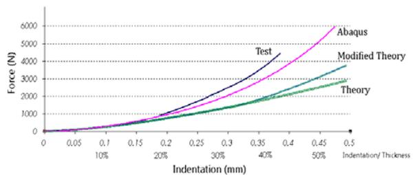
Fig. 10 Indentation in 4layer laminates with 20mm indentor
