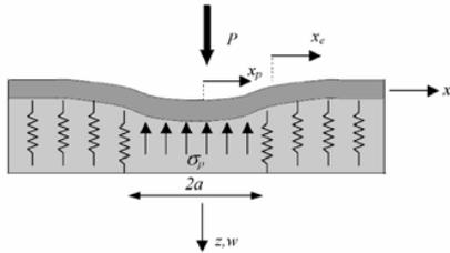
Fig. 11 Indentation model of sandwich beams [9]
