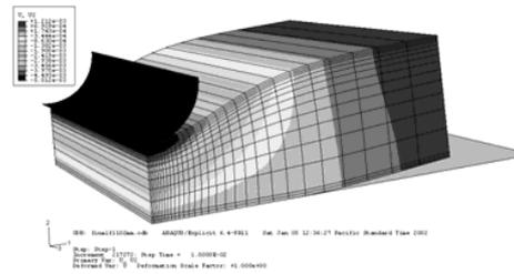
Fig 13 Indentation modeling of sandwich beam in Abaqus
