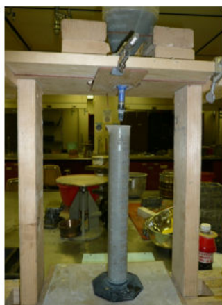
Fig. 1 Modified marsh cone test (MMCT) apparatus and the results of the paste mixes made of W/B ratio of 0.3
