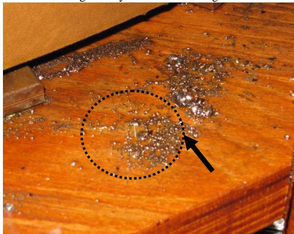
Fig. 11: Eroded copper chips
