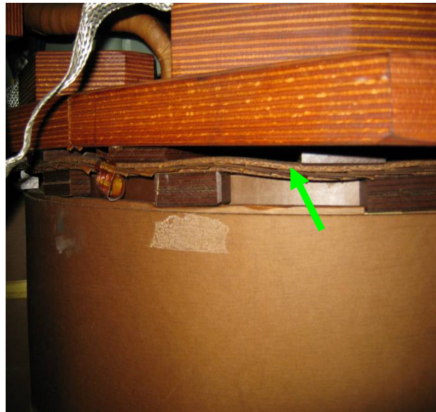
Fig. 8(a): Wavy pressboard due to coaxial force
